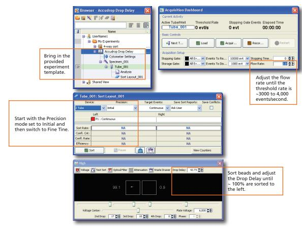
Open your sorting experiment and set up the Sort Layout.
