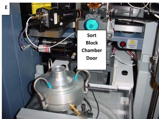
Figure E. Impactor placement. Top of collection chamber.
