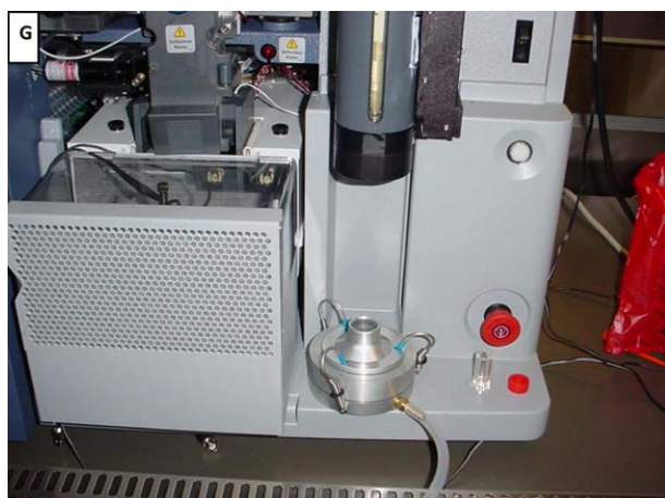
Figure G. Impactor placement. Under sample station.
