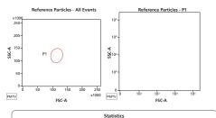
An example of a worksheet used to acquire unstained cells and adjust PMTVs until the target rSD values (2.5 x rSD<sub>EN</sub>) are reached.
