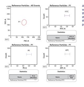
An example of a worksheet used to verify that MFI values for stained cells fall within the linearity of each parameter.
