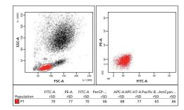
An example of a worksheet used to acquire unstained cells and adjust PMTVs until the target rSD values (2.5 x rSD<sub>EN</sub>) are reached.
