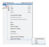
b. A template may also be created and shared across instruments with identical configurations. Right-click the experiment, and select
