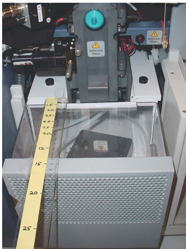
Figure 1. Photograph of aerosol measurement locations on top of FACS Aria collection chamber. Samples were taken on top of the collection chamber at the indicated locations. For measurements taken at 20 and 25 cm, measurements were taken at the same relative height as closer measurements.
