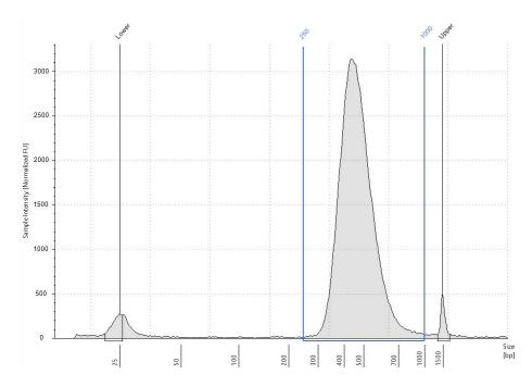
**NOTE** If smaller products (~165 bp or ~270 bp) are observed in Figure 3, such as the peaks shown in Figure 4, a second round of AMPure XP magnetic purification is recommended. See Additional WTA Index PCR purification steps in the following section.
