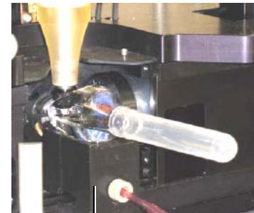
Debubble reservoir located on the flush bucket during a wet shutdown
