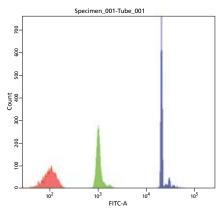
Cytometer Setup and Tracking beads are excited by all supported lasers and emit in the range of virtually any filter combination.
