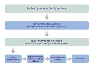
BD<sup>TM</sup> Cytometer Setup and Tracking Beads, designed for use with BD FACSDiva<sup>TM</sup> 6.0 or later software, automate the characterization and tracking of BD FACSCanto<sup>TM</sup>, BD FACSCanto<sup>TM</sup> II, BD FACSAria<sup>TM</sup>, and BD<sup>TM</sup> LSR II flow cytometer performance. The bead reagent vial contains sufficient volume and concentration to perform 50 daily performance checks or up to 16 baseline characterizations.
