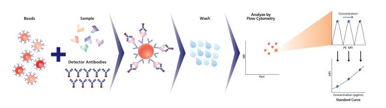
A BD<sup>™</sup> Cytometric Bead Array (CBA) assay contains a cocktail of beads bound with specific capture antibodies that differ slightly in fluorescence intensity. The beads are mixed with samples along with PE-labeled detection antibodies and run on a BD Accuri C6. BD CBA can analyze 300 beads per protein—the equivalent of 300 ELISA wells—for up to 30 cytokines simultaneously. In essence, BD CBA is like running multiple ELISAs at once using flow cytometry.
