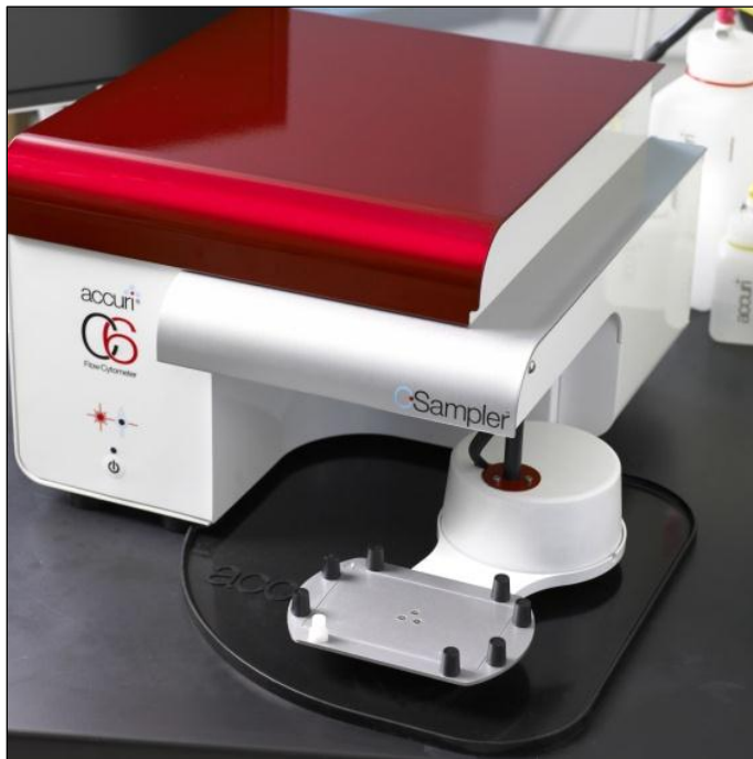
Figure 1-8. BD CSampler with Mat Installed
