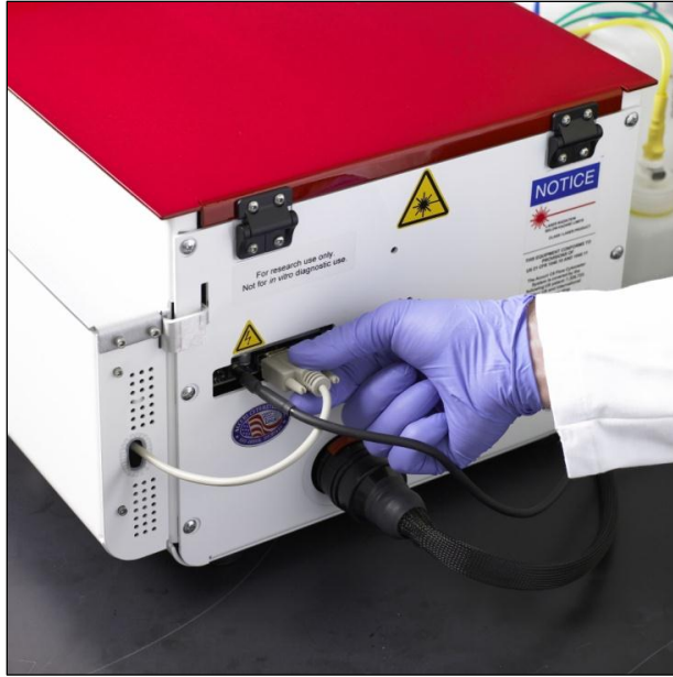
Figure 1-7. Connect the BD CSampler Cable to the Flow Cytometer
