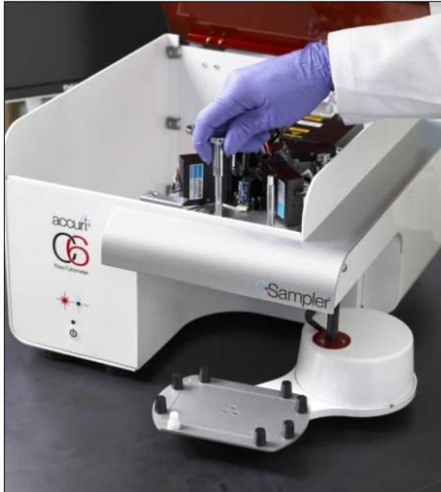
Figure 1-6. Secure the BD CSampler to the Flow Cytometer
