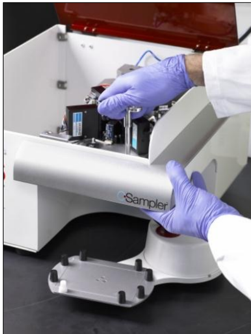
Figure 1-5. Secure the BD CSampler to the Flow Cytometer
