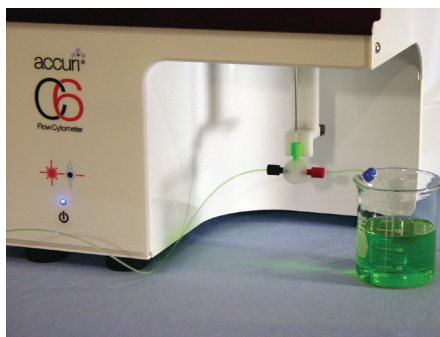
Figure 6. The tee connection from the FlowCytoPrep to the BD Accuri C6 SIP. The cytometer takes the amount of sample it needs and discards the rest into a waste reservoir.
